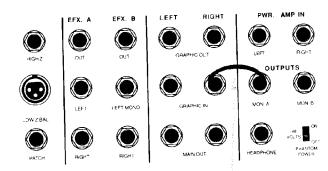
PATCH MONITOR A OUTPUT INTO RIGHT GRAPHIC INPUT
