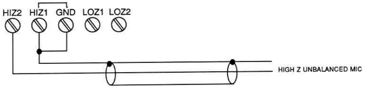
Figure 7. High Z, Unbalanced Microphone Input Connections
