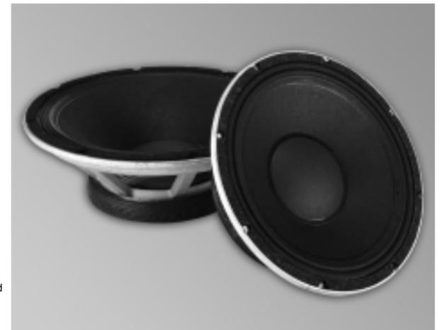
The voice coil assembly is bonded to the Kevlar cone and new super-tough nylon composite spider using a thermoset epoxy originally developed for attaching nose cones on ICBM missiles – truly an aerospace-grade adhesive. The spider and surround are bonded to the frame with a high strength toughened-cyanoacrylate adhesive, which is also used to bond the dust cap to the cone.
