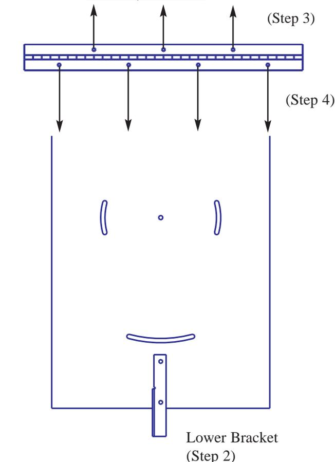
Step 5. Position the midrange horn and plywood base assembly right side up on top of the low frequency speaker cabinet. Align the four pivot holes and slots in the base with those in the speaker cabinet. Loosely install four 1/4" x 1 1/4" machine bolts and flatwashers through the base into the low frequency cabinet.
