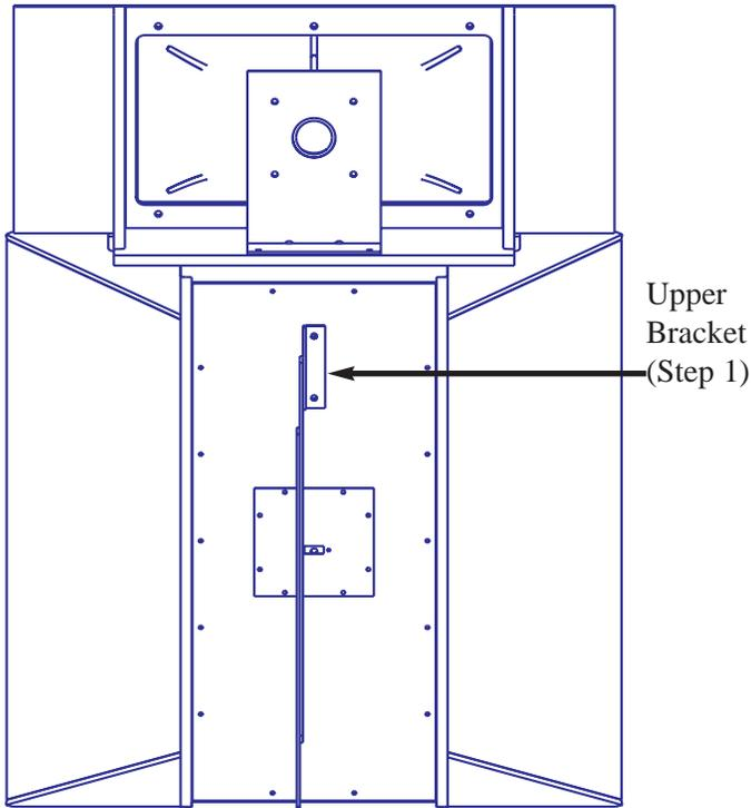
Step 1. Install the upper bracket to the midrange horn as shown with two 1/4" x 7/8" machine screws and flatwashers. With the horn right side up, the protruding flange with the center hole of the upper bracket will be on the left when facing the cabinet back.
