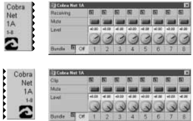
Fig. 18, CobraNet Input and Output Controls (Bundle Numbers in the OFF position)
