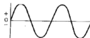
ALTERNATING VOLTAGE APPLIED TO PLATES OF DIODES
