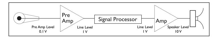
The audio chain begins with the microphone. A microphone is a device that changes energy from one form to another. A device that changes energy from one form to another is called a transducer. The microphone is a transducer that changes acoustical energy (sound) into electrical energy (voltage). The acoustical energy may be the sound of someone's voice or that of a musical instrument.
